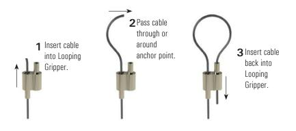
**Notes:** Minimum 2" cable to exit bottom of gripper when done. Remove load before adjusting.
