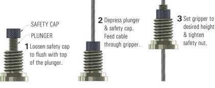
**Notes:** Minimum 2" cable to exit bottom of gripper when done. Remove load before adjusting.
